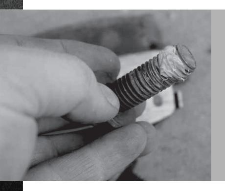
Threadlockers are designed to prevent loosening of nuts, bolts and assemblies from shock and vibration and seal threads against rust and corrosion. VersaChem® offers two types of anaerobic thread lockers -Threadlock Formula Type 245 for frequent disassembly and easy removal and Stud & Bearing Formula 275 for those projects that require a longer, stronger seal.
